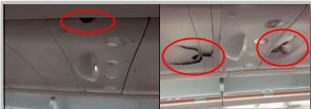
Figure 4. Damage on passenger service units
